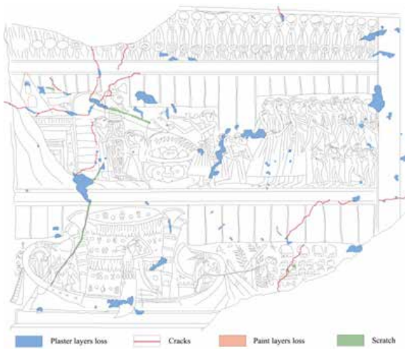
図17 Zone E の損傷図面 Fig.17 A result of condition survey at Zone E
